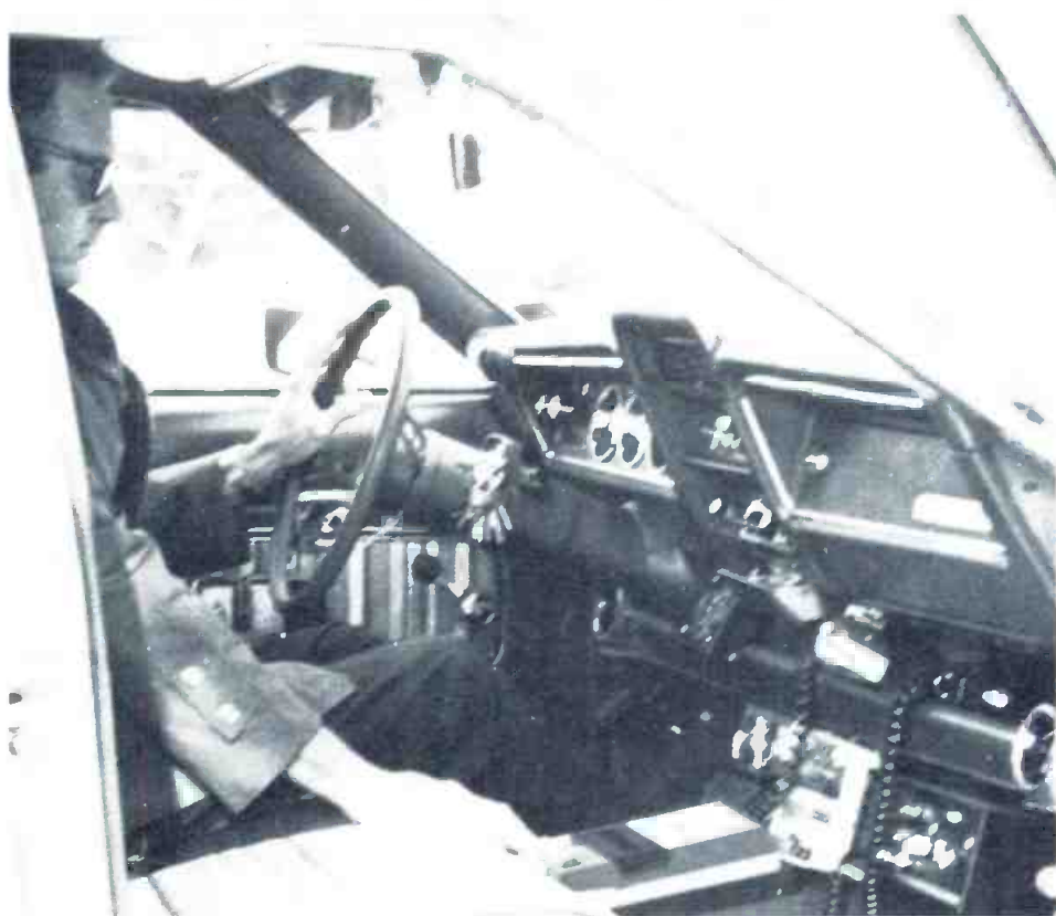
The cassette recorder is mounted on the transmission hump where it can be easily reached. Also visible is the 2 Meter FM gear at right.
